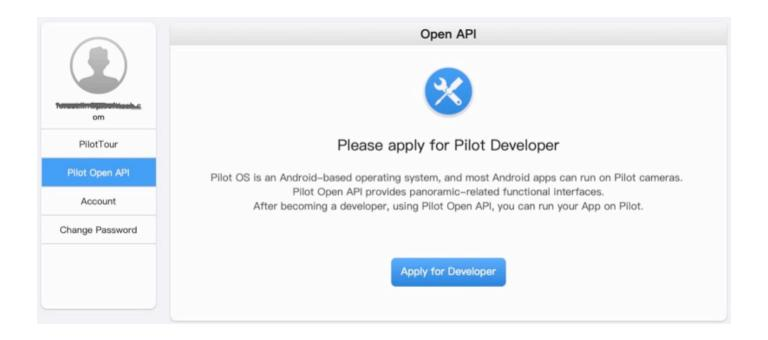
After becoming a Pilot developer, open Pilot, enter Settings - Pilot ID - Open API, the USB debugging mode will automatically turned on, and developers can install and debug their own apps on the Pilot.
