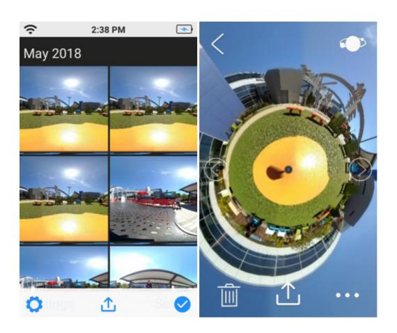
Tap a photo/video to enter playback view. In playback view, double-tap the screen or tap the icon in the upper right corner to switch the view mode. View modes include: Little Planet, Equirectangular, Fisheye, and Rectilinear.
