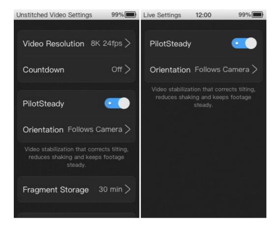
PilotSteady has two orientations: Fixed, Follows Camera.
